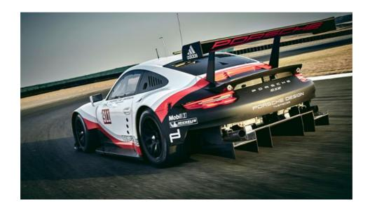
The new 911 RSR makes full use of the breadth of the Le Mans 24 Hours GT regulations, and in addition to systematic lightweight design, features the ultra-modern, flat-six unit positioned in front of the rear axle. The four-litre, extremely light aggregate features direct fuel injection as well as a rigid valve drive and is characterised by outstanding efficiency. The new 911 RSR will make its debut at the Daytona 24-hour race in January 2017.
