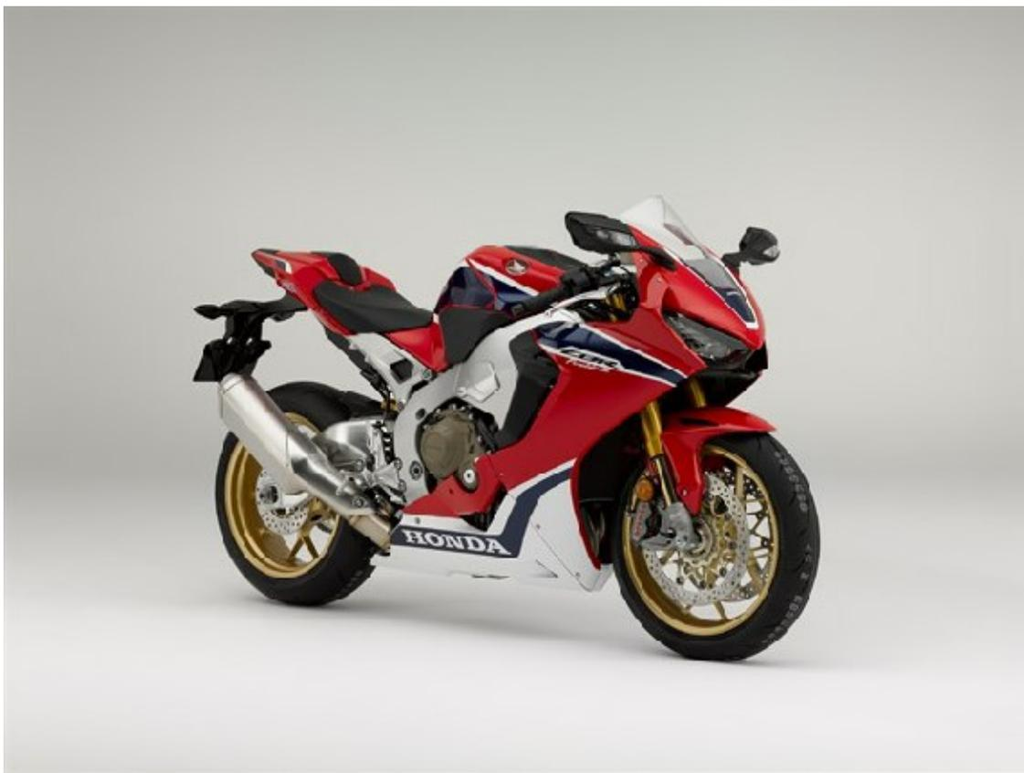
Visually the carbon pattern insets and gold striping interwoven into the Tricolour paint mark the Fireblade SP2's difference over the 'stock' machine and gold Marchesini wheels (reducing front/rear wheel inertia by 18/9%) are another clue. But the real differences – and what gives the Fireblade SP2 ultimate racing potential – lie inside the engine and, in turn, the parts that can be added from the two race kits that will be available.
