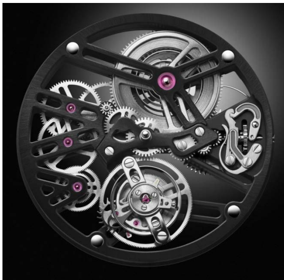
Manufacture Angelus A-300 calibre Tourbillon movement with optimized beam-type bridges and Angelus six-spoke design wheels for maximum stiffness and weight saving © ANGELUS SA
